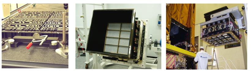
**IBIS** (Ubertini P., Lebrun F., Di Cocco G., et al, 2003, A&A 411, L131) is optimized for high-resolution (12'), wide FOV (29°x29°), point sources imaging and moderate energy resolution (8% @ 100 keV, 10% @ 1 MeV). It is composed of 2 detectors:
