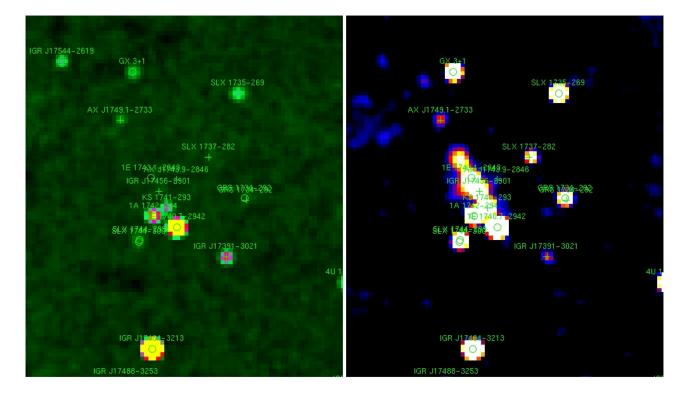
Is your source of interest variable, transient or steady? A "variability map" (left) could help: each pixel of the map is the  $\chi^2$  of the fit of the ScW- by- ScW lightcurve by a constant. Variable sources appear bright on the variability map.
